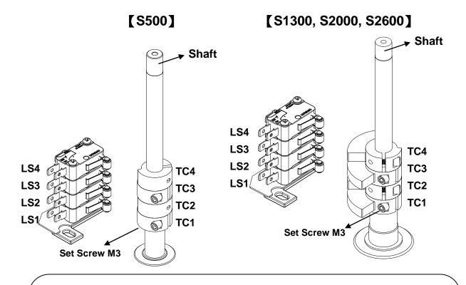
TC 4 Synchronous turn with TC2 (option).TC 3 Synchronous turn with TC1 (option).
