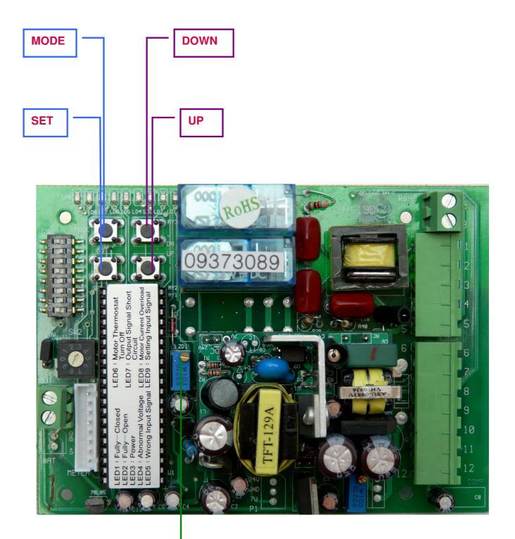
VR2-Feedback adjustment (10V or 20mA) Output feedback signal The users don't need to set 2V or 4mA
