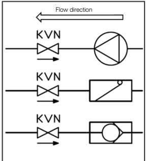
Direction of installation in front of the components
