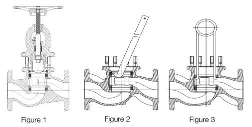
11.2 Checks during Valve Ring Replacement
